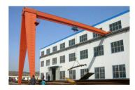
Semi-gantry Crane has a special design structure to suit various crane work situations. It can be single girder and double girder, the two ends connections are different, one side is connected and supported by the crane gantry leg travel on the ground mounted rails, another side is connected and supported by an end carriage travel on the overhead track.
