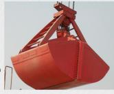
The four-rope grab is mainly used with bridge or gantry cranes with two sets of lifting drums to grab all kinds of loose deposits, and perform operations such as loading, unloading, and transferring materials. Mainly supporting double girder bridge crane or double main girder gantry crane.
