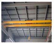
LH type electric hoist double beam crane is traveling on fixed support, the frame adopts box-type welding mechanism, and it used together with CD1 or MD1 model wire rope electric hoist as a complete set, It is an mid-duty class crane, the capacity from 3 tons to 20 tons. The span is 10.5-31.5m. Working class is A3~A4. Working temperature is -20°to 45°centigrade.
