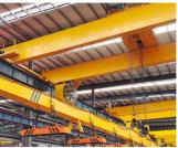
The crane is mainly equipped with electromagnet, When the current is turned on, the electromagnet will firmly attract the steel objects and lift them to the designated place. Cut off the current, the magnetism disappeared, and the steel object was put down. The crane is suitable for scrap recycling plants and steel mills.
