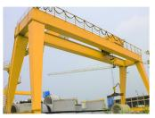
The European-style gantry crane is designed and manufactured according to the advanced standards of European Standard Co., Ltd. Its rated capacity is 3 ~ 20t. The lifting mechanism is a European-style electric hoist trolley. The trolley is equipped with a reducer and a three-in-one transmission.
