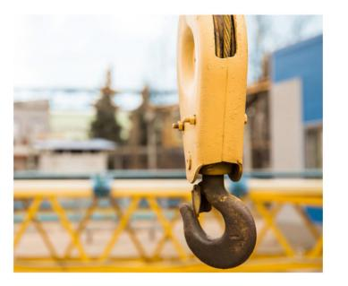
Industrial hoist hooks is one of the most suitable slings in hoisting. It is connected with pulleys to hang on the wire rope of lifting mechanism. And the hook is the most widely usage when lifting cargos. It is made easily and operated practically.
