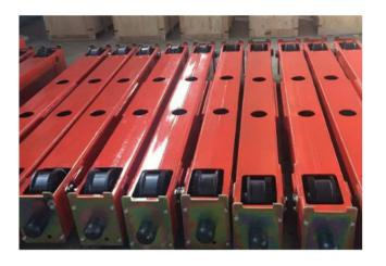
Single Beam End Beam For Bridge Crane is composed by Wheels, motors, buffers, collector base, girder joint plate and bolts, etc. The end beam adopts rectangular control, CNC boring and milling integrated customized machine tool, a one-time completion of opening, boring, drilling. Equipped with high quality reducer, hollow shaft drive, high working level, wide speed adjustment range, widely popular.
