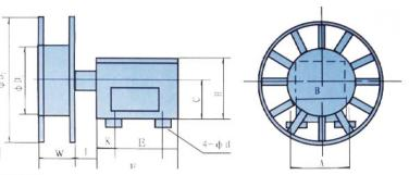
Motor cable reel is a winding device used for large mobile starting equipment to transmit power, control power, or control signals between two relatively moving bodies. It is widely used in heavy machinery equipment such as port gantry cranes, container cranes, ship loaders, tower cranes, and other similar working conditions.
